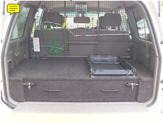
Std 2 Drawer, S/S Water Tank, Cargo Barrier Fridge slide to suit Engel 40, Waeco 50 lt
