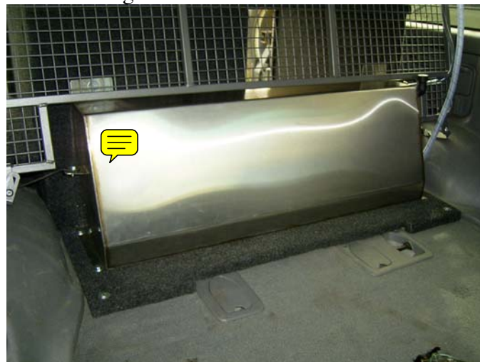
60 Lt S/S Water tank, Special Half Cargo Barrier behind FridgePack 3 drawer – Seats not affected
