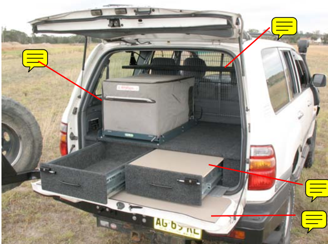
Std 2 Drawer, Engel 60, water tank, Cargo Barrier Cargo barrier shelf, tailgate table, drawer top table
