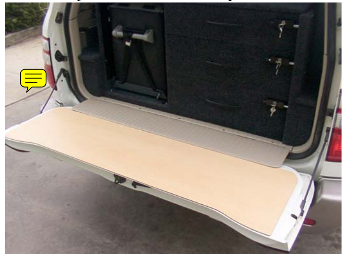
Tail Gate Table – Replaces original carpet liner Laminex top NO Screws required
