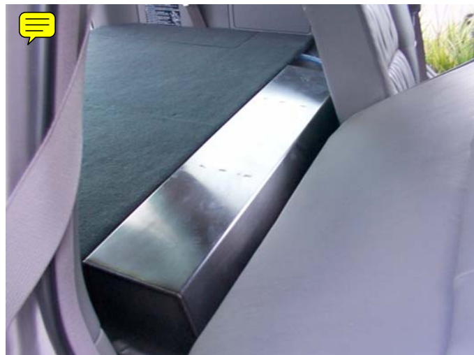
45 Lt stainless Steel Water Tank behind standard 2 drawer
