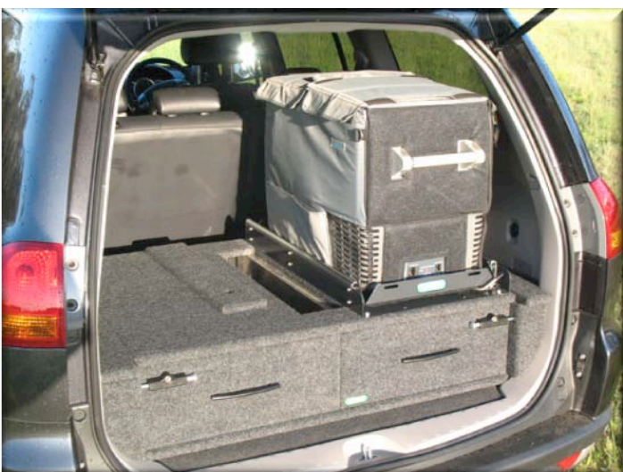
Centre hatch cover allows easy access to the spare tyre winndown mechanism. It is also a handy place to store tools and spares.
