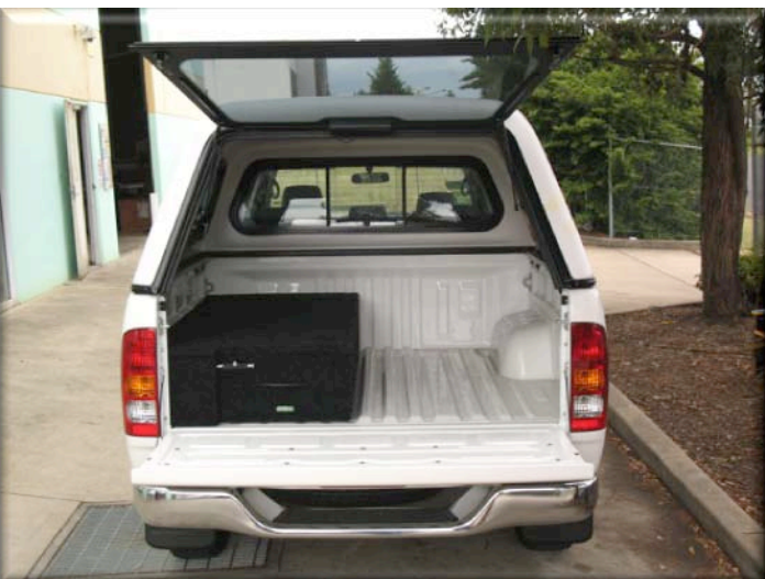
A Single Drawer fitted over to one side still allows larger items to be placed into the tray on the other side.
