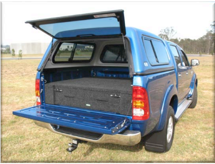
“Long 2 Drawer Aluminium” . There are wing panels on the side of each drawer that lift up to allow access to the storage area behind the wheel arch.
