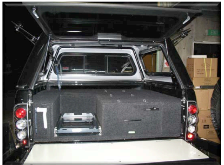
Custom single drawer system with optional stainless steel water tank, rear pump and tap setup, laminated tailgate table and stainless steel eye bolts to tie to.
