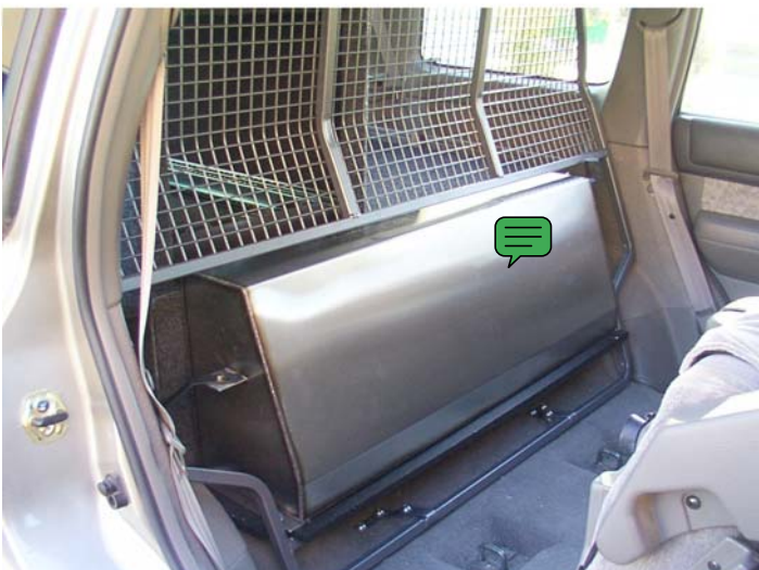
60 litre Stainless Steel Water Tank & Special Cargo Barrier mounted in front of standard 2 drawer
