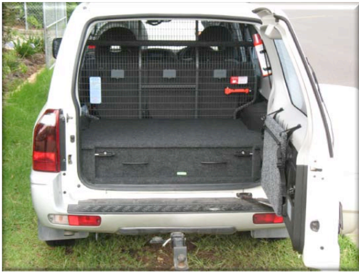
“Aluminium Standard 2 Drawer” with an optional full height “Ausguard” cargo barrier and a “Cargo Barrier Storage Shelf” fitted.
