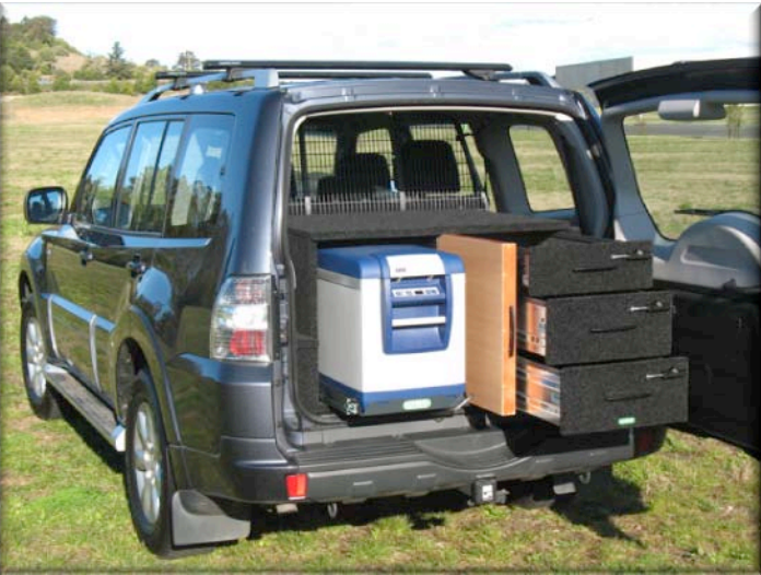
We use high quality ball bearing runners on all of our drawers and fridge slides. It makes for an effortless and rattle free operation.
