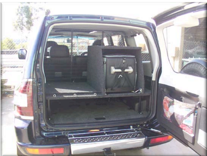
ORS “Storage Platform” with an optional “Fridge Slide” and “Fridge House”. These create easy access to your under floor storage bin without the need to unload your fridge or extra cargo.
