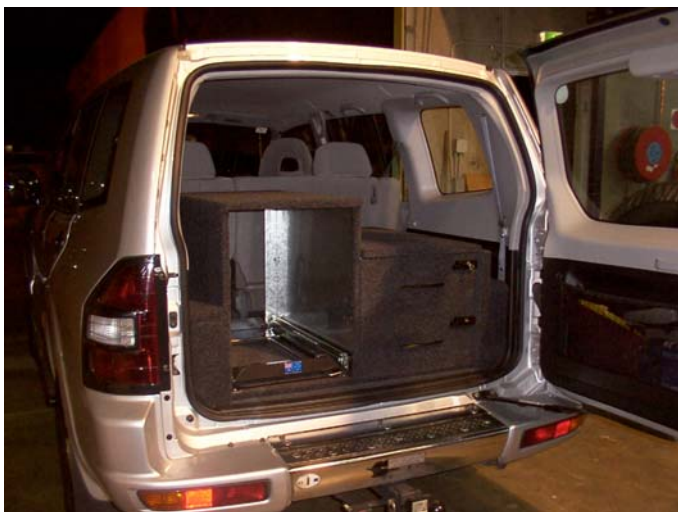
Fridgepack 2 Drawer Medium, Fridge compartment to suit Engel 40 lt, Waeco 50 lt, Bushman 42 lt
