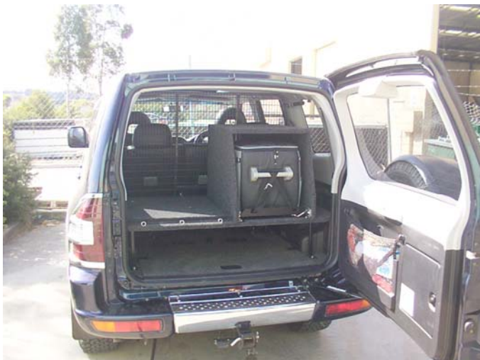
Special Platform under Fridge unit to access Seat well after seats removed
